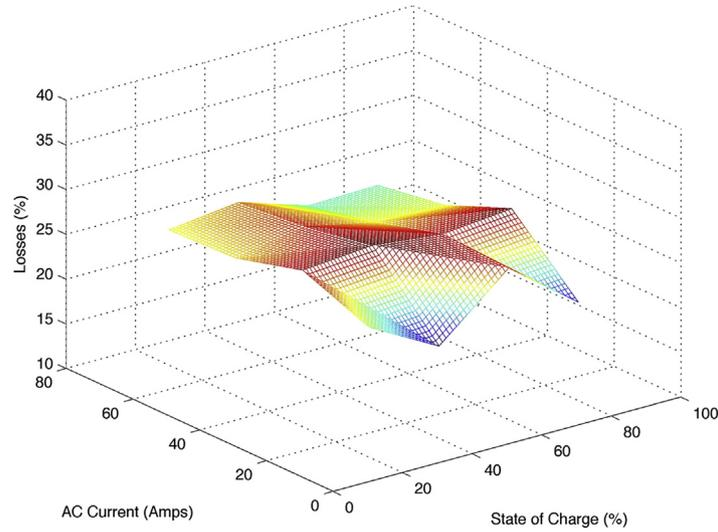
Fig. 3. Interpolation of round-trip losses (PEU and Battery).
